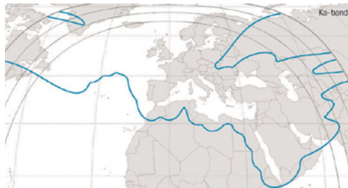
Telenor's Thor 7 satellite will provide Ka-band coverage over the North Atlantic, Europe and the Middle East
